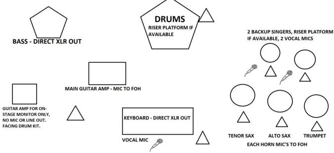
SMALL TRIANGLES = WEDGE MONITORS INPUTS = 3 VOX MICS, 3 HORN MICS, 1 GUITAR AMP MIC. DRUM MICS AS DETERMINED BY FOH. XLR DIRECT OUT BASS, KEYBOARDS
